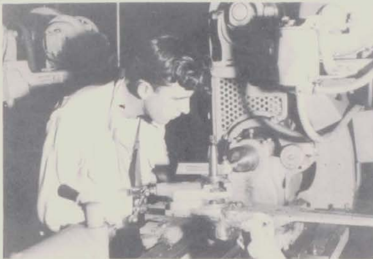
Robert Hanson turns small details for a surface gauge.
