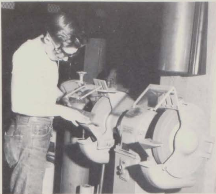
George Paulson does a grinding exercise on lawn mower blades.
