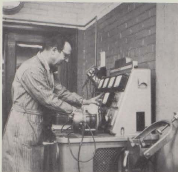
Peter Aldo, automotives instructor, manipulates a generator and regulator tester.
