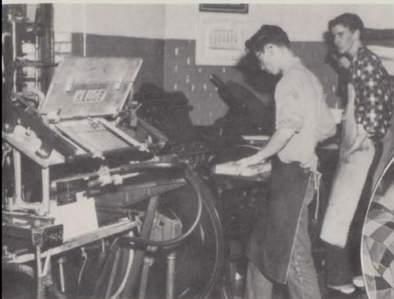
As future printers Larry Price, Robert Shaw, and George Girdley operate a Platen printing press, the Kluge press does its job automatically.
