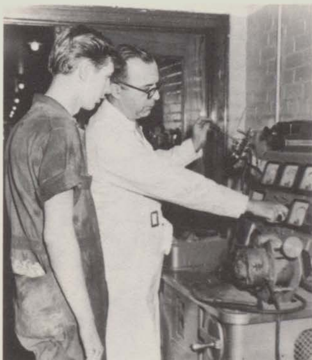
Pete Aldo, Pontiac Central's automotive instructor, demonstrates the Generator Regulator Test Bench to Dick Young. Facilities such as this give students a chance to learn by experience how to operate automotive machines.
