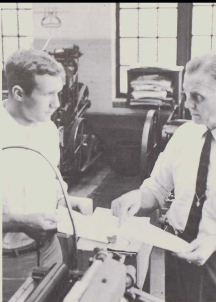
The Multilith duplicating machine, used in printing letterheads and bulletins, is part of the modern photo off-set process. Instructor Ted Carlson shows examples of the work produced by the machine to Al Galbraith.
