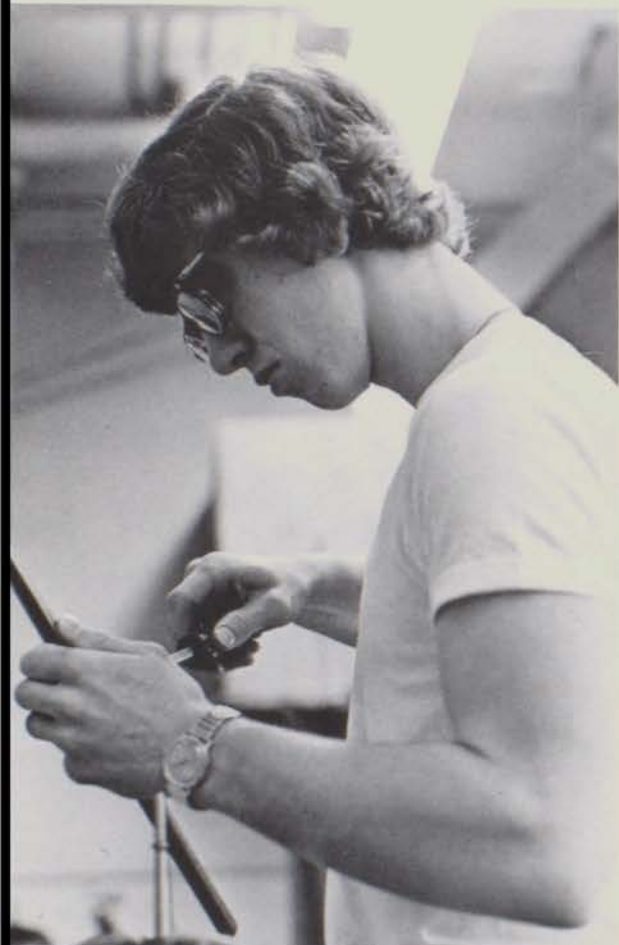
WITH HIS MIND TUNED TO WORK, Peter Montney installs a tapping device into a tapping wrench before beginning the assignment.
